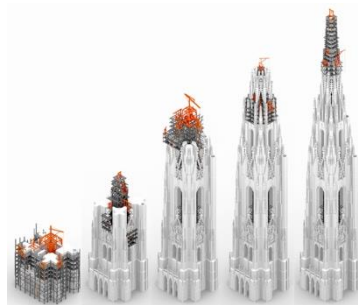
Fig. 18. The five main phases of a Gothic tower's construction. Drawing by author.
