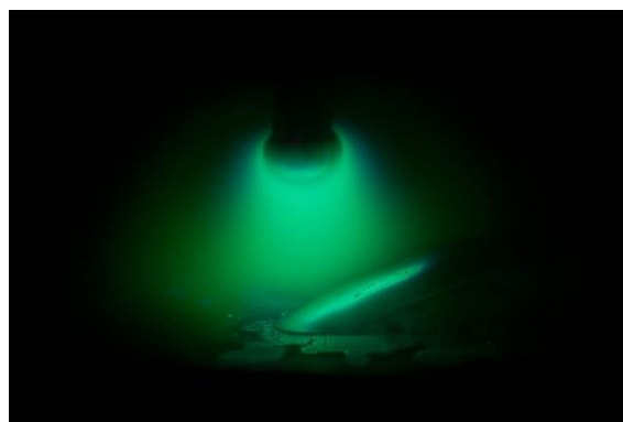
Fig. 13. Metal drop at the filler wire tip
